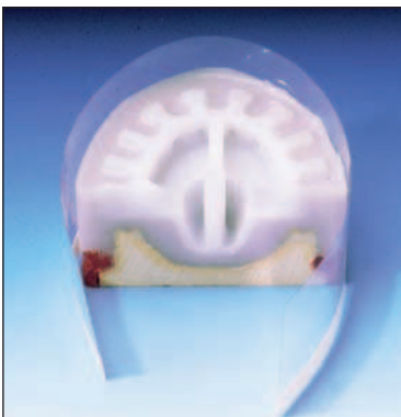
Cross-section of a flaskless duplicating mould
