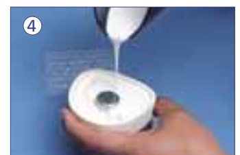
4 After positioning the magnet holder and magnet pour the secondary base.
