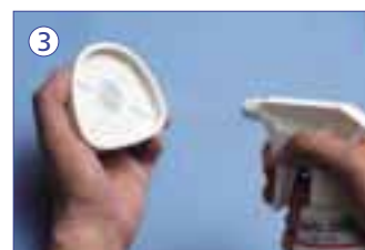
3 Isolate plaster against plaster
