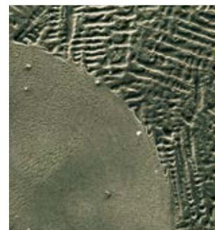
Laser weld without any cracks in a carbon-free CrCoMo alloy
