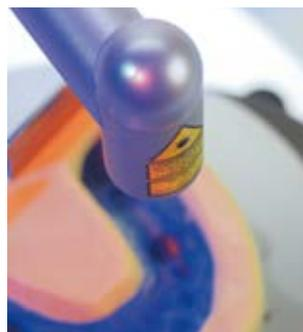
Laser beam for easy drill positioning
