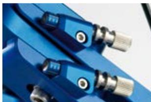
A easy and highly precise setting of the enlargement factor is feasible by making use of the micrometer screw
