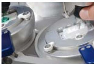
Easy processing of undercuts by tilting the spherical shell table
