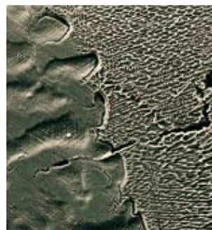
Cracks caused by carbide precipitation in a CrCoMo alloy containing carbon
