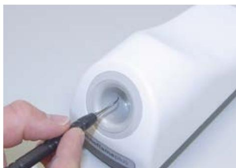
Within seconds, the modelling instrument is heated in the coil opening
