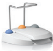
Chiropro foot pedal Pedal with 3 buttons and variable speed drive. Functions: progressive speed, ON/OFF peristaltic pump, program selection, selection of the micromotor's direction of rotation. For iChiropro, Chiropro L and Chiropro control units. Ref. 1600631-001
