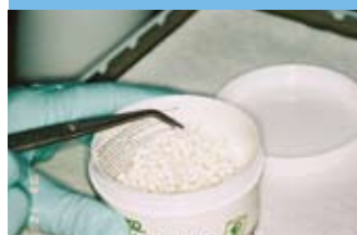
Cylindrically shaped etching pellets for use with etching gels and pastes
