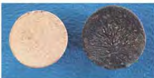
In this picture the difference between casting the same alloy in natural atmosphere and casting in inert atmosphere is evident.
