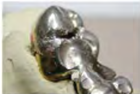
Welding with alloy addition
