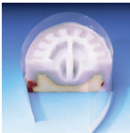
Cross-section of a flaskless duplicating mould
